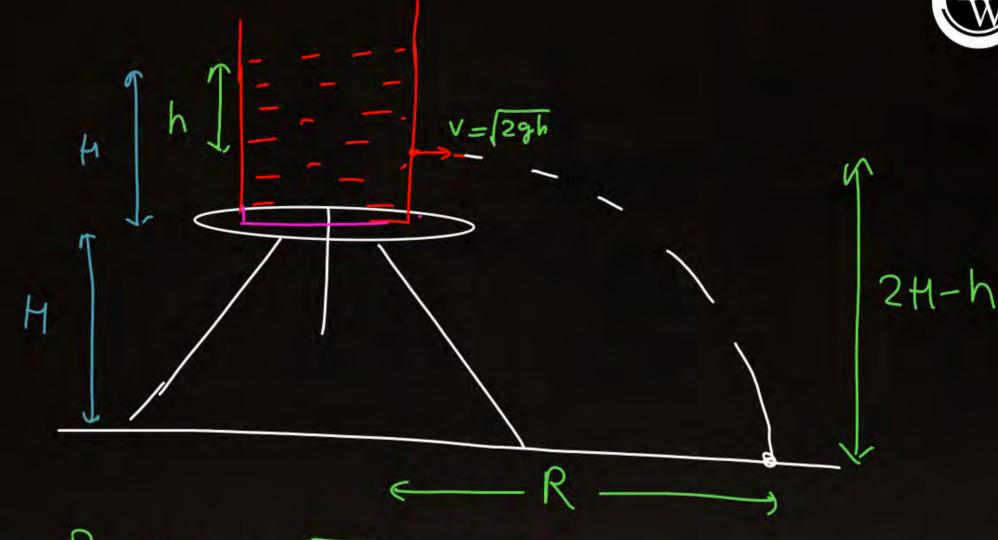
24. A vent tank of large cross-sectional area has a horizontal pipe 0.12 m in diameter at the bottom This holds a liquid whose density is 1500 kg/m³ to a height of 4.0 m. Assume the liquid is an idea fluid in laminar flow. In figure, the velocity with which fluid flows out is:
